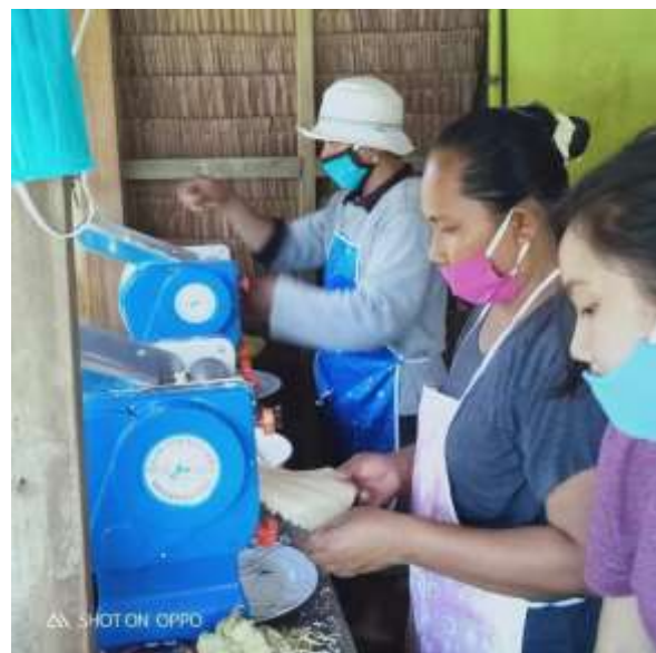
Assigned member of BUDLIS fisherfolk organization make raw squash noodles with a machine extruder, then weigh it per 50 grams prior to boiling and drying. PHOTO COURTESY OF CERD-BANTAYAN BAY PROGRAM
